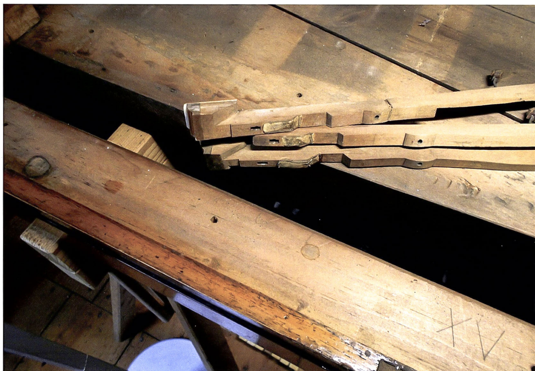
Illus.3 Showing the gap in the baseboard for the organ trackers, and the leather pads under the keys for contacting the trackers
