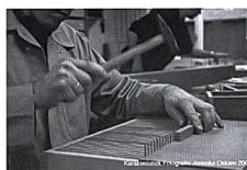
Technicians making guidepins for a wind chest
